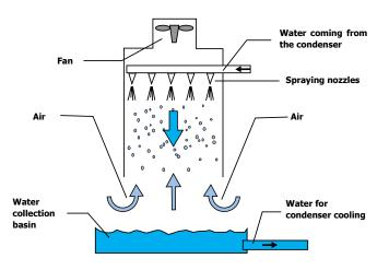
Therefore, in the case of evaporative towers, while air enters from below, induced to rise by the fan or by the difference in density, the water to be cooled is sprayed from above. This will have a high temperature at the entrance, as it has previously received heat from an environment, from an engine or from any component. In contact with colder air, the liquid sprayed into the tower releases energy, partially evaporating and cooling according to the principle set out above.
